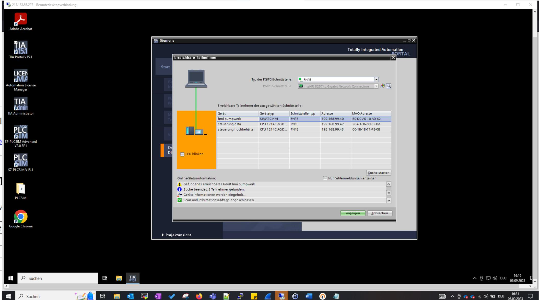
The screenshot shows a remote desktop connection to a Siemens TIA Portal V15.1 workstation. The main window is titled "Erreichbare Teilnehmer" (Reachable Participants) and displays a table of discovered devices connected via a PN/IE interface. The table lists three devices: "hmi pumpwerk", "steuerung dsta", and "steuerung hochbehälter".
